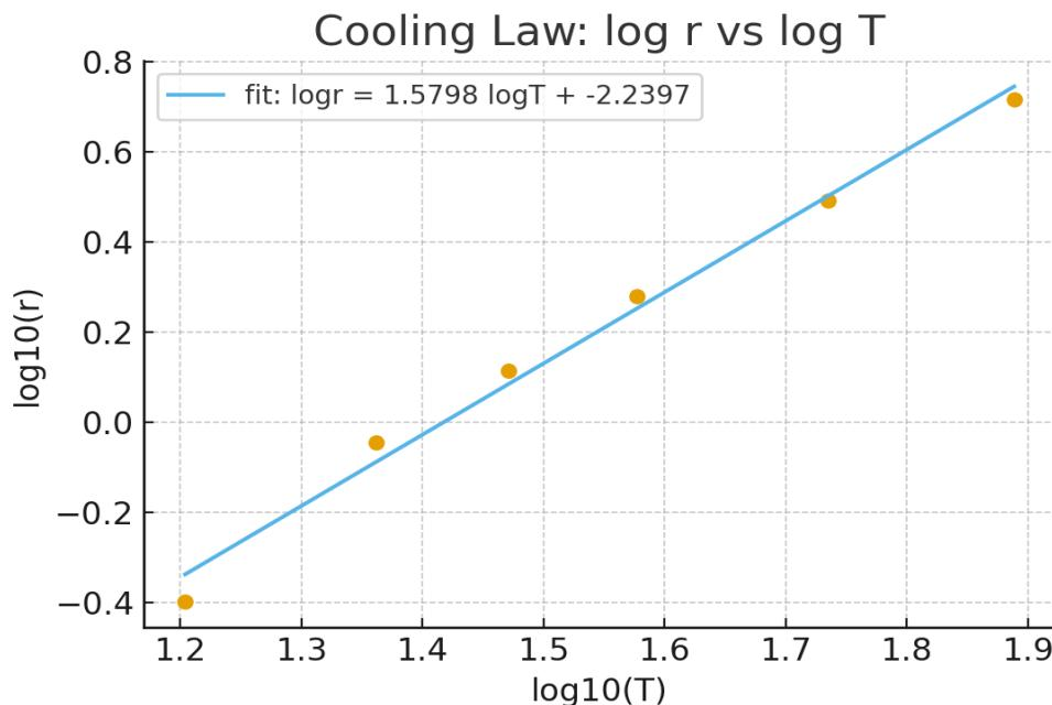
Result of linear fit:  $\log r = n \log T + \log a$  with  $n = 1.5798$  and  $\log_{10}(a) = -2.2397$ . Therefore  $a = 3.0000$ .
