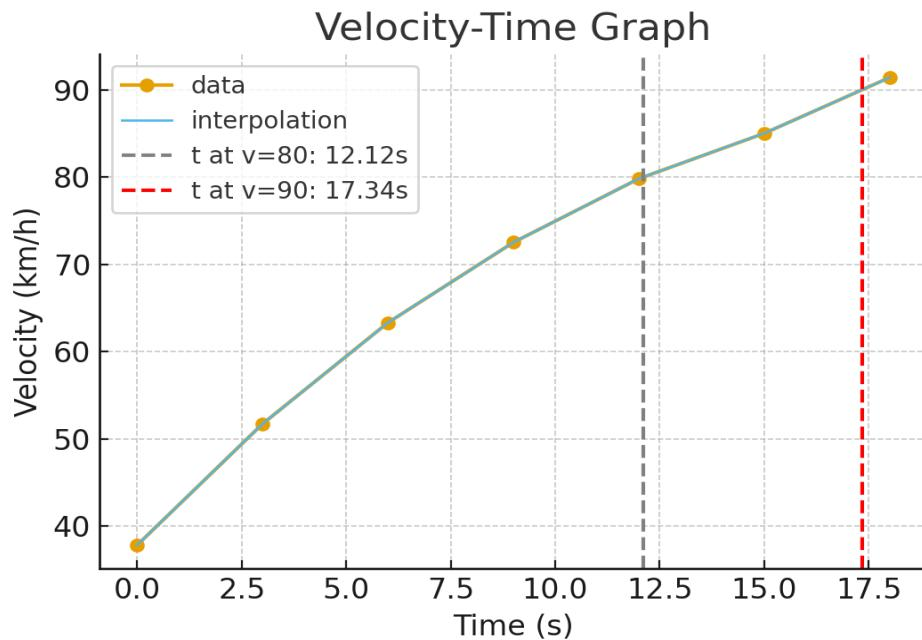
(a) By linear interpolation on the velocity-time curve we find time at  $v=80\text{ km/h}$ :  $t = 12.12\text{ s}$  and at  $v=90\text{ km/h}$ :  $t = 17.34\text{ s}$ .
